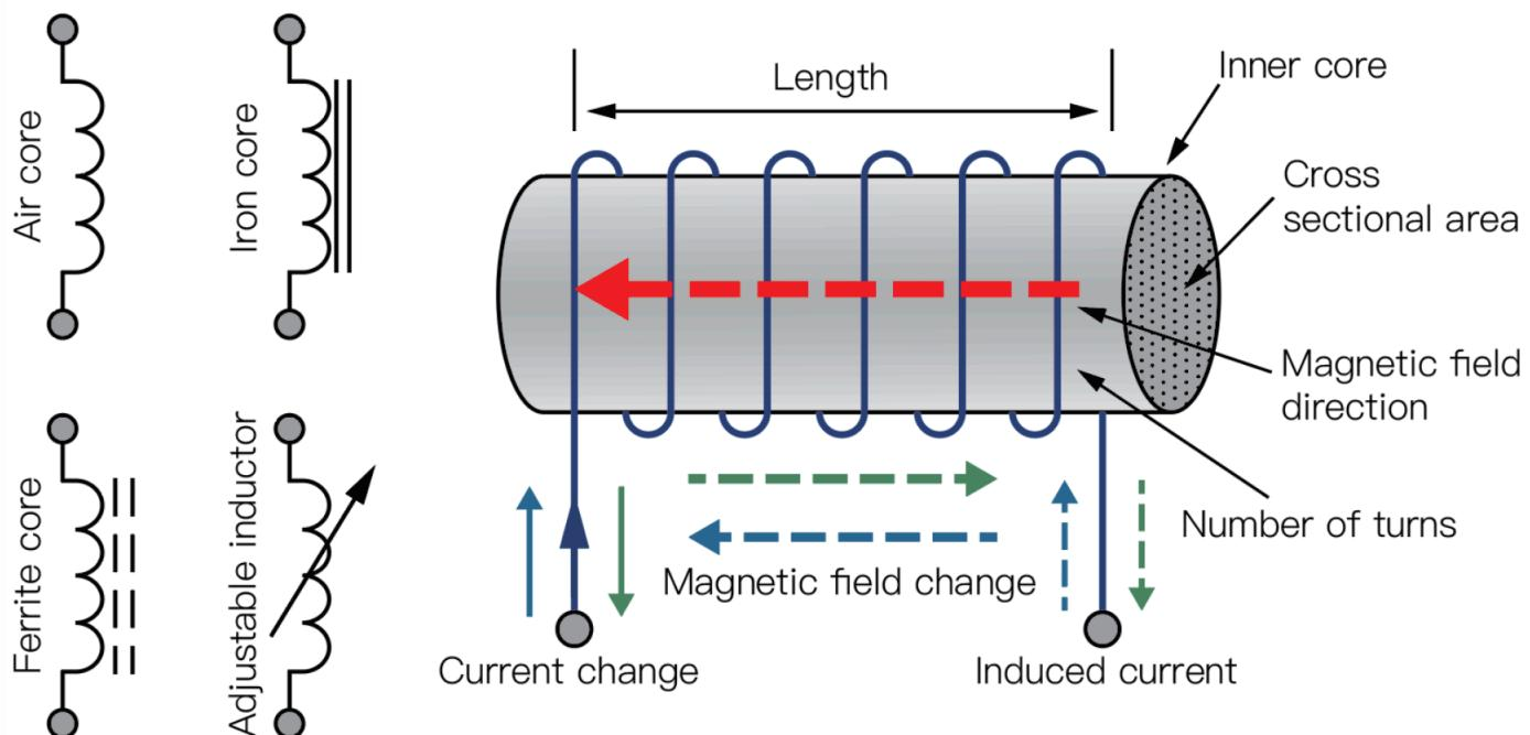
In electronic circuits, inductors serve a wide range of purposes, which has led to the existence of numerous types. This article briefly presents the methods for selecting inductors.
